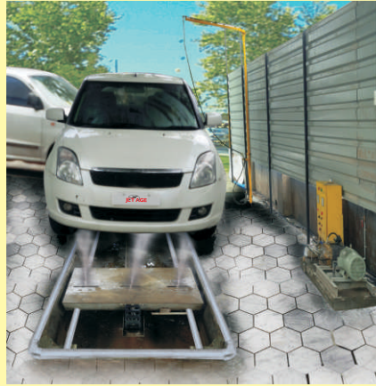
Under Body Wash Plant
